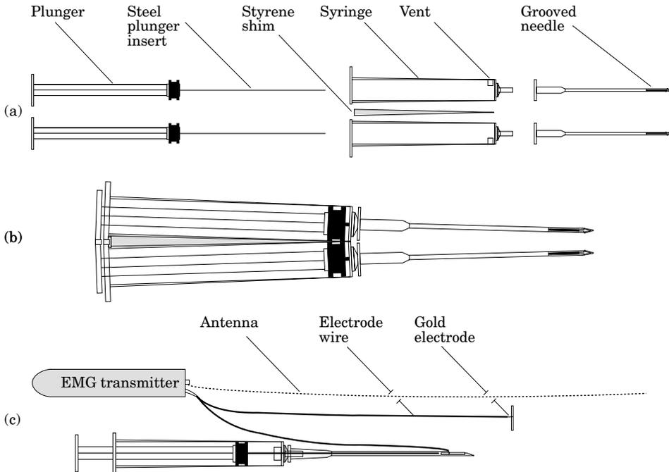
FIG. 1. (a) Components of the tool used to facilitate implantation of EMG electrodes (exploded view). (b) Assembled tool (plan view) with syringe and shim held together with hot glue. (c) Transparent lateral view of the implantation tool showing EMG electrode loaded into needle groove.
