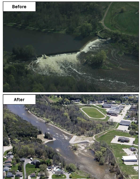
Figure 1 – Aerial images of the Truax Dam footprint, Walkerton, ON, before and after removal. The original wooden dam was built in 1852 and later replaced by the concrete structure shown above in 1919. While the dam had a fishway that allowed the passage of some migrating salmonids under specific flow conditions, it posed a significant barrier to fish passage before it was removed to restore river connectivity.
