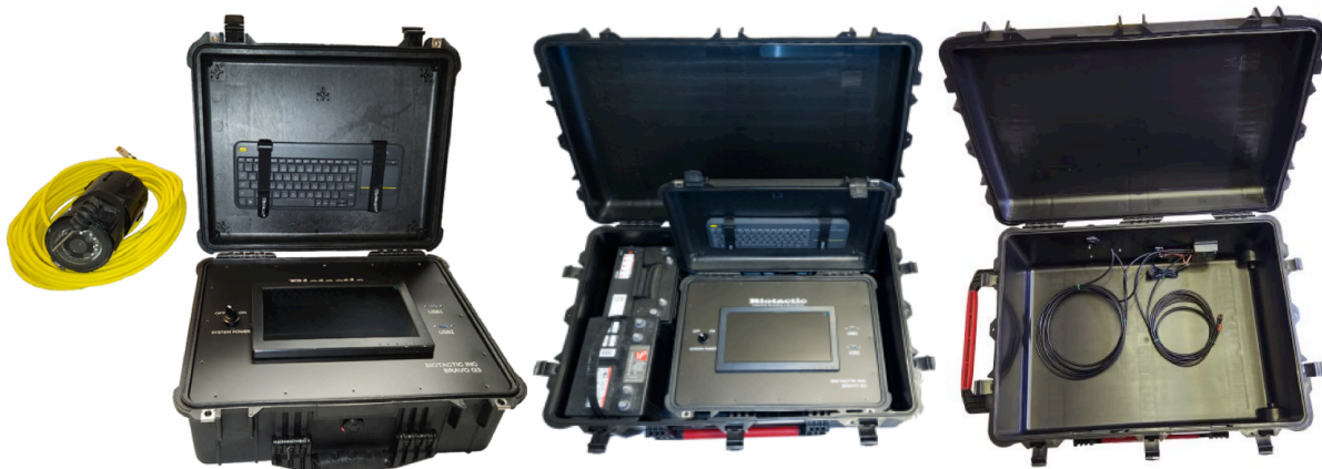
Figure 1. BRAVO G3 systems can be operated using solar panels and 12V deep-cycle batteries in remote locations. This requires an additional power unit case. The power unit case is shown above (right) - dimensions (inches) 32 length x 23 wide x 16 height. The left image shows only the G3 system plus camera and cable, and the middle image shows the G3 system inside the power case with batteries.
