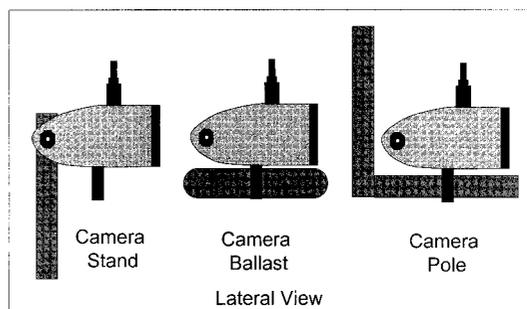
FIGURE 3.—Variety of underwater camera deployment configurations. A camera stand can be devised by using thin metal such as aluminum (described in text). Camera ballasts provided with the camera can be used for down-rigging or other applications that involve towing the camera at depth. Poles can be devised to position the camera as desired for exploratory or stationary monitoring.
