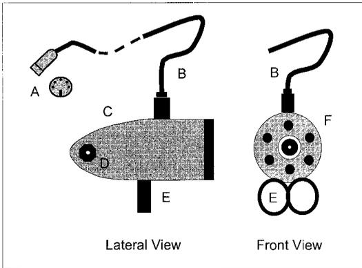
FIGURE 1.—Schematic of the camera we modified for use in fisheries research. The camera interface, a 5-pin Deutsche Industrie Normenausschuss (DIN) plug (A), is plugged into C (Figure 2). The cable (B) connects permanently to the main camera body (C). An attachment mechanism (D) provides opportunity to attach a fin or camera stand. Ballast weights are secured into (E). A frontal view of the camera (F) illustrates the six LEDs and the central location of the camera lens.
